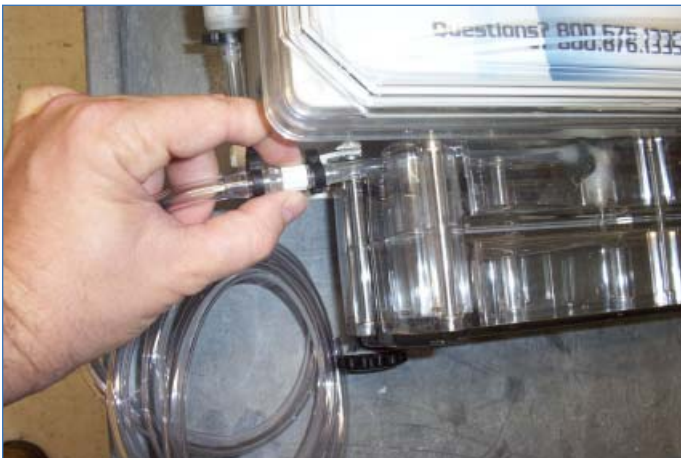
Figure 15 - Acid Injection line
