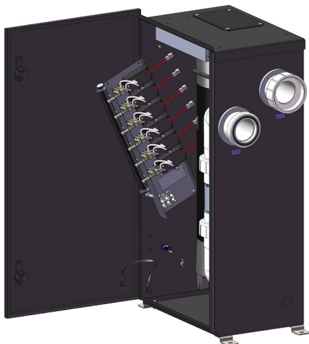
Figure 6: Ozone Bracket During Ozone Module Service
